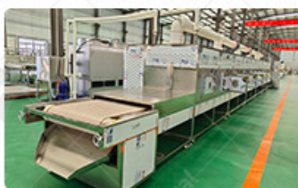
6. Machine Material : 304 stainless steel
