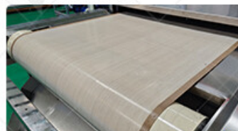
3. Belt: Customizable meshbelts of various materials
