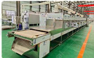
6. Machine Material : 304 stainless steel
