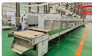
6. Machine Material : 304 stainless steel
