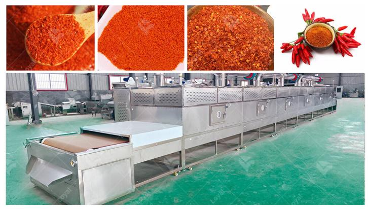
The Chili Powder Microwave Sterilization Machine is tailored for precision in the sterilization process. Utilizing microwave technology, it offers a controlled and uniform heat distribution, effectively eliminating any potential contaminants in the chili powder. The machine's design ensures that the spice's flavor, aroma, and nutritional content remain intact, meeting the highest quality standards in the food industry.
