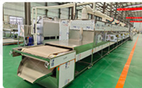
6. Machine Material : 304 stainless steel
