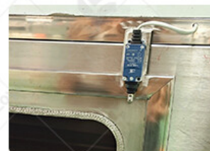
5. The observation window is equipped with a travel switch to prevent microwave leakage and improve safety.
