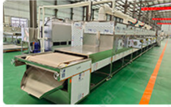
6. Machine Material : 304 stainless steel
